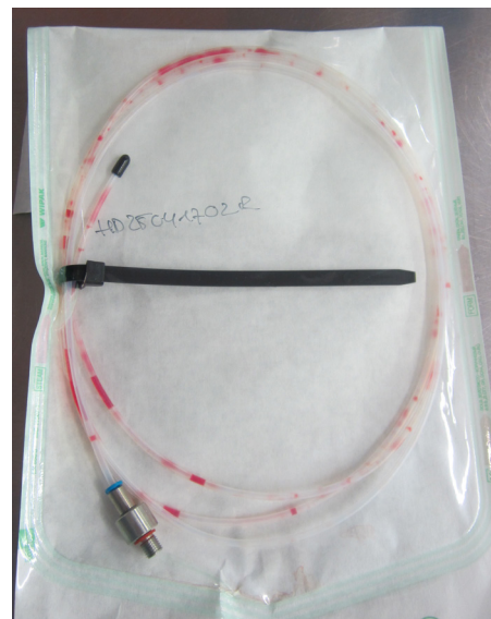
Fig. 1. Test tube after standardized contamination.
