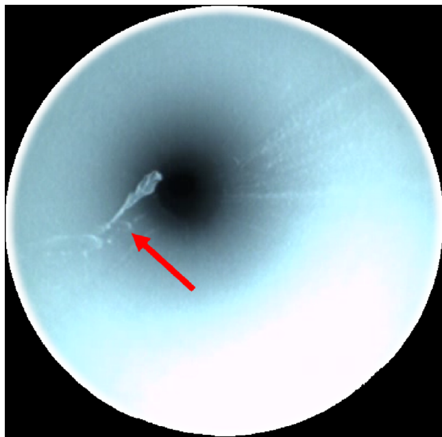
FIGURE 5 Scratches in the endoscopic channel (indicated by red arrows).
