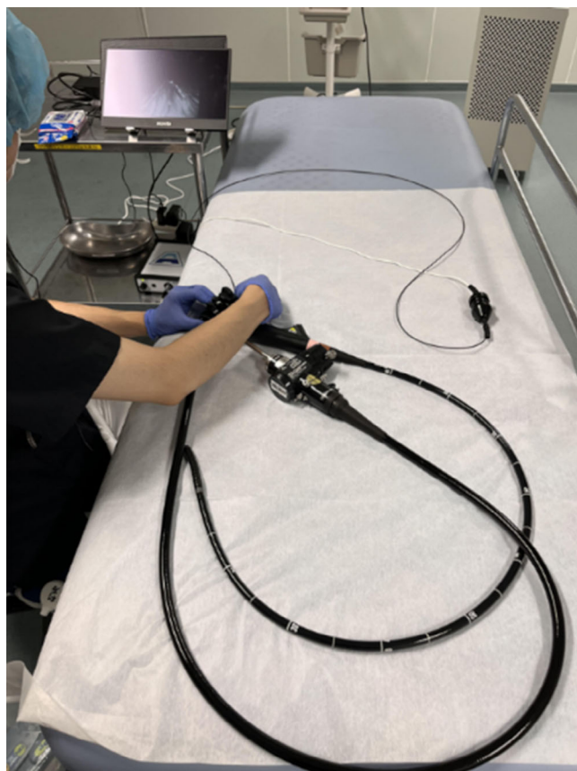
FIGURE 3 Actual observation of the lumen of an endoscope using EYEBOSCO.
